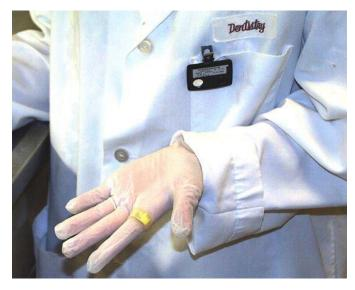
The dosimeters do not protect a worker from radiation exposure. They will not provide any visible or audible warning when being exposed to radiation. They are essential, however, in tracking a worker's radiation dose and confirming that occupational dose limits are not exceeded.
